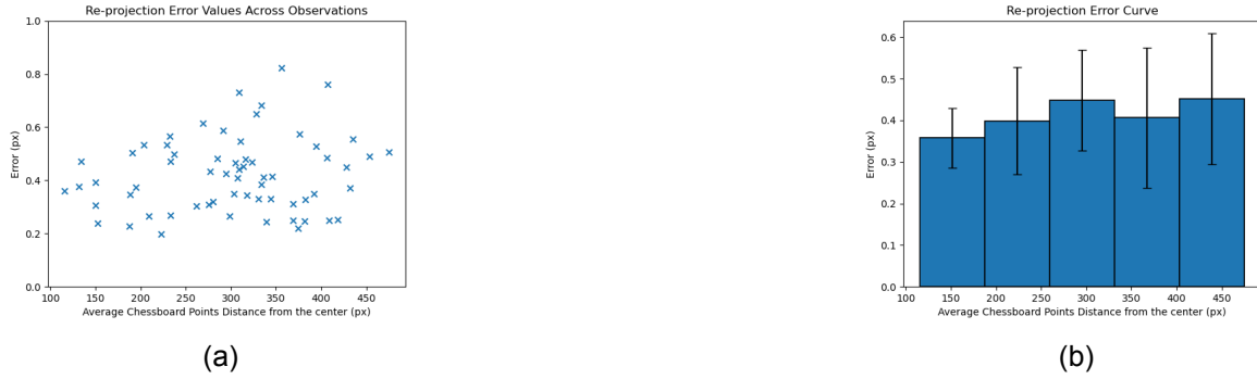
Figure 5.8: Re-projection Error Values ( px ) vs. Average Chessboard Points Distance from the centre ( px ) as a Scatter Plot (a) and histogram (b).
