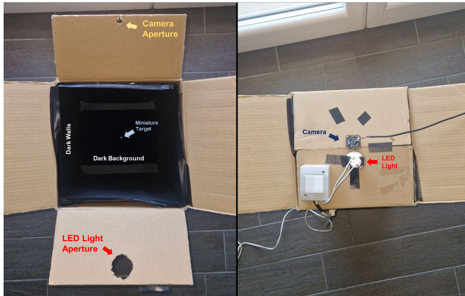
Figure 6.1: Experimental Cardboard Box Dark Room Setup (miniature over-size).
